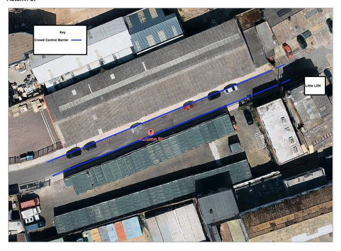
The external barrier placement on Autumn Street will be used to create a segregation between the footway and highway to eliminate obstruction to the highway for vehicular access as well as for pedestrian safety.
